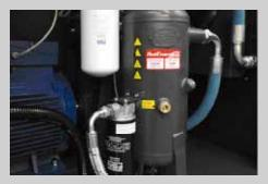
**Oil filter and oil separator filter** Both spin-on type, ensure maximum efficiency and ease of maintenance.
